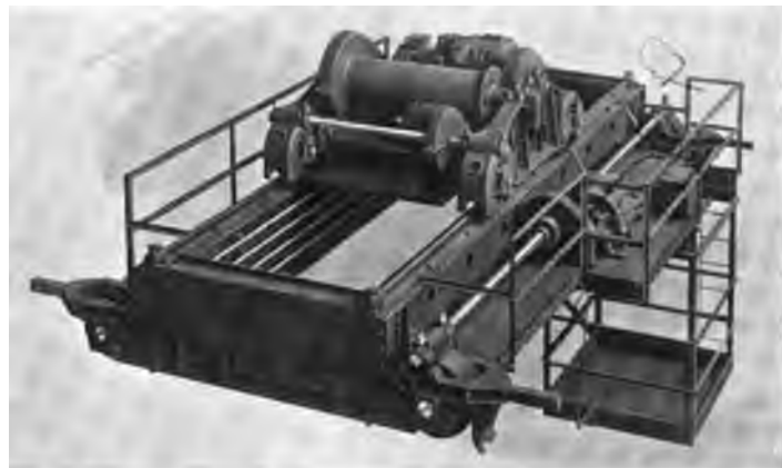
Fig. 4. Traveling Crane with Excellent Arrangement of Gear Guards, Walks, etc.
